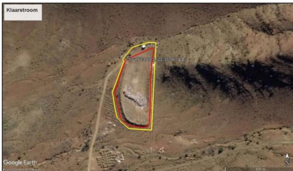
Based on the used footprint, 1:4 side slopes and a height of 3m at the southern edge, the available airspace was calculated as 3, 877m<sup>3</sup> with use of the topographical survey of June 2022.
