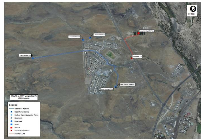
Figure 4.8: Water Infrastructure in Bitterwater/ Leeu Gamka
